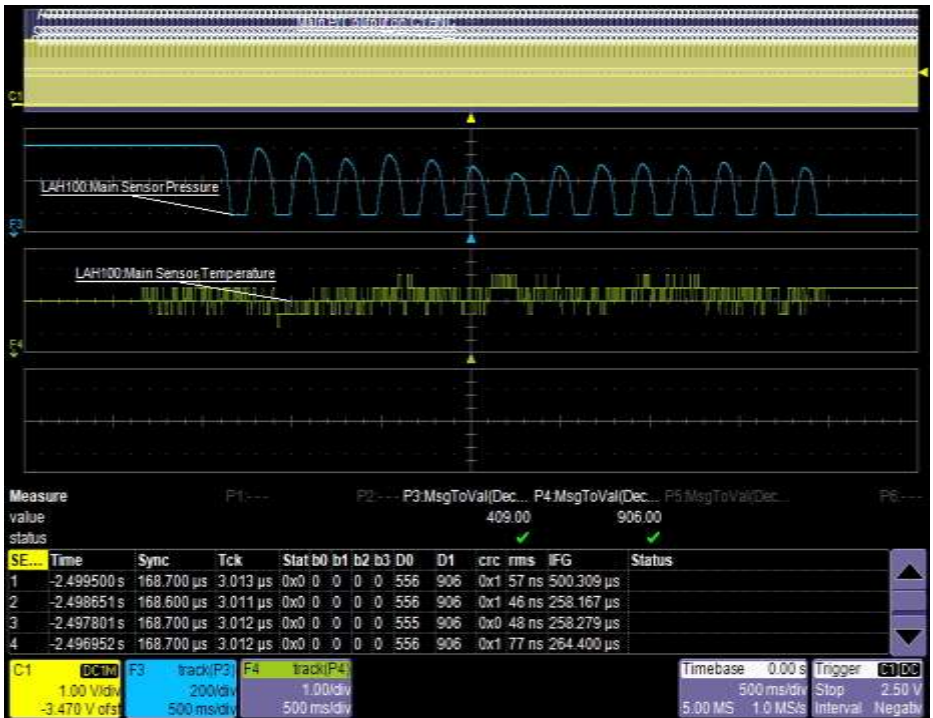
Figure 17 Track of P and T on the sensor over a time span of 5 seconds
