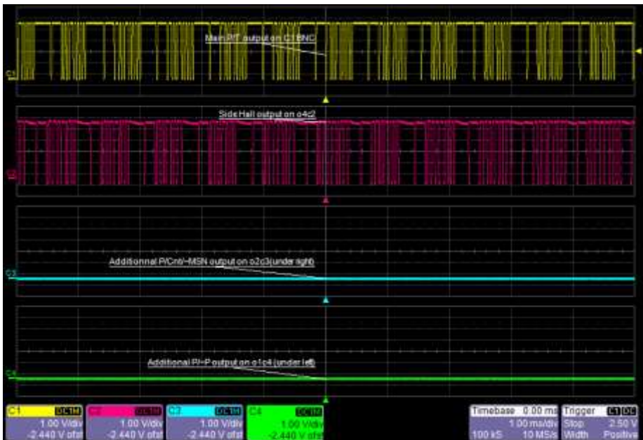
Figure 10 Basic Functionality Test of LAH100, showing the SENT activity
