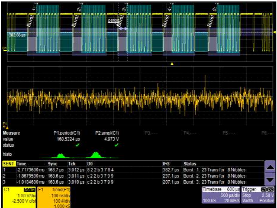
Figure 11 Monitoring Stability of the TickTime, with a SYNC of 168.5 μs
