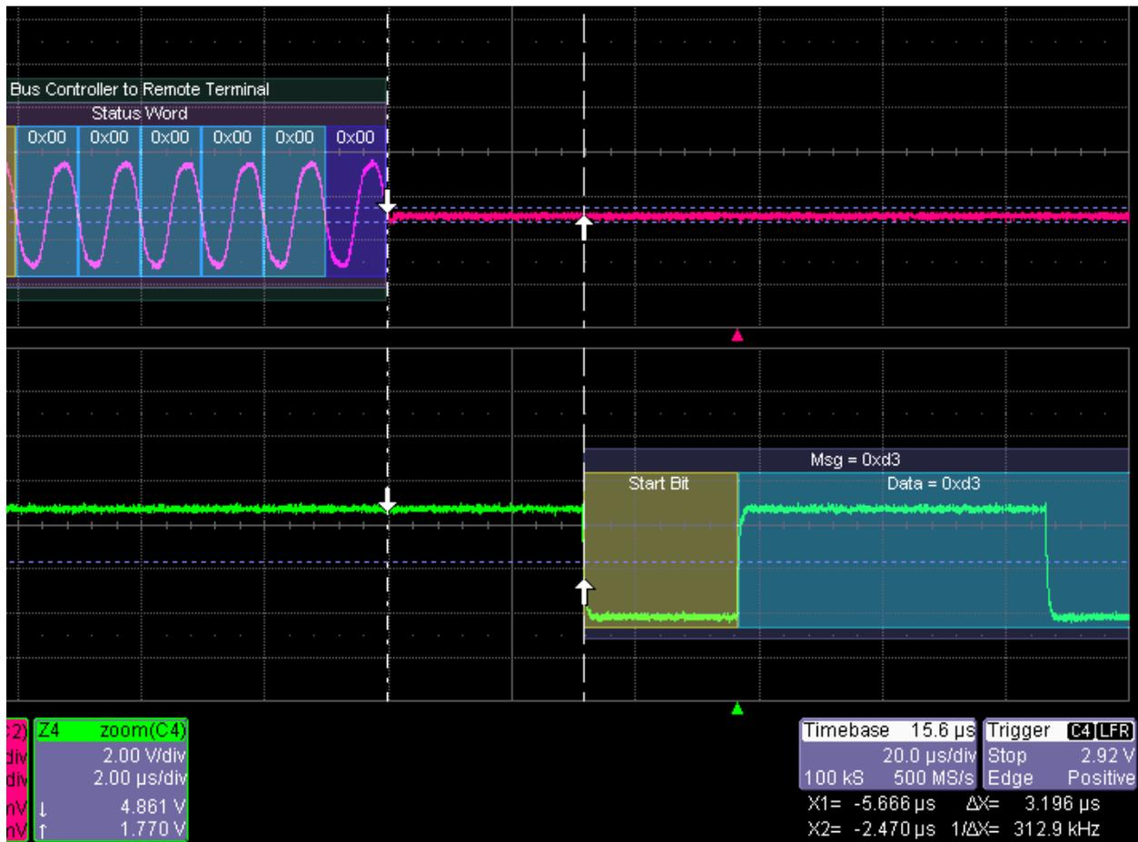
Figure 4: Shown here is a zoom of Figure 3. The synchronous acquisition on all channels permits observation and measurement of the time difference between the end of the MIL-STD-1553 message (end of the parity bit) to the beginning of the UART message (beginning of the Start Bit). The time lag is measured as 3.196 microseconds.
