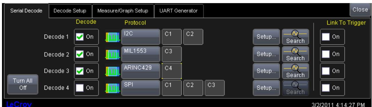
Figure 1: The User Interface exhibits an array of 4 Decoders, each one with the appropriate inputs (Data, Clock, Chip Select), analog or digital. The setup tabs of each decoder adjust dynamically to the selected protocol.
