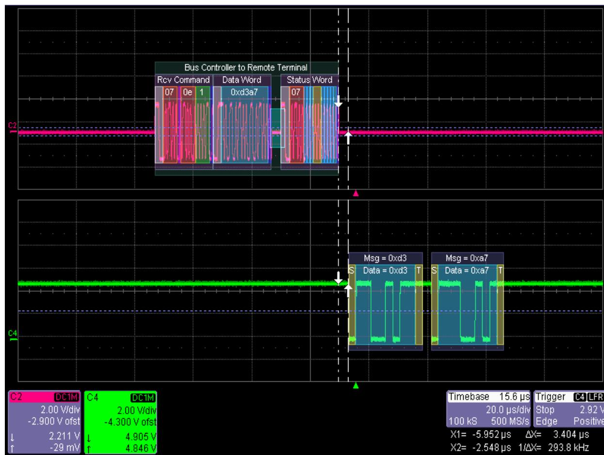
**Figure 3: An example of a MIL-STD-1553 (1 Mb/s, Manchester) bus on Channel 2, inducing a UART message (400 Kb/s, NRZ) on Channel 4. The approximate translation latency of 3.4 microseconds is read out using the cursors. The data word 0xd3a7 on the CAN bus is split into 2 words on the UART bus.**
