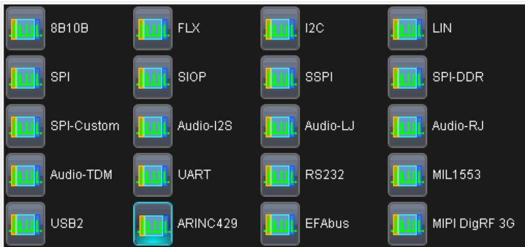
Figure 2: Protocol selection popup, with a variety of serial streams used in different application domains.
